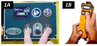
To use the optional Remote Control System, hold the <u>"function" button</u> ( 1, fig. 1B) and the <u>"release" button</u> (  $|\rightarrow\rangle$ , fig. 1B) on the <u>radio transmitter</u>.
