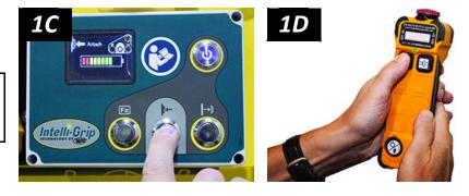
To use the optional Remote Control System, press the <u>"attach" button</u> ( ↓←, fig. 1D) on the <u>radio transmitter</u>.
