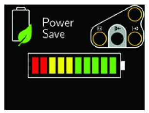
along with a diagnostic code (see "INTELLI-GRIP® DIAGNOSTIC CODES" on page 31). In this case, you must charge the battery in order to continue using the lifter.
