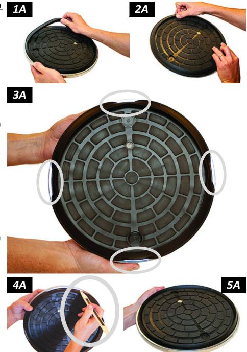
5) Make sure the sealing ring seats securely in the mounting groove, all the way around the vacuum pad (fig. 5A).
