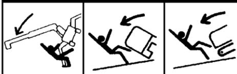
When the machine inclines in excess of 3 degrees during crane work, or in excess of 15 degrees during travel, the tipping alarm buzzer will sound. For preventing it from tipping over, return it to the state for the buzzer not to sound at once, and start the work or traveling.
