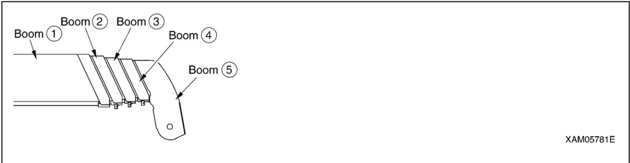
2. “Boom (1) + (2)”: With booms (3), (4), and (5) retracted, boom (2) is fully extended.
