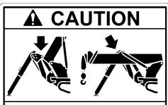
The boom may hit the outrigger in crane work, by depending on the state for the outrigger to have been extended.
