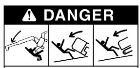
When the machine inclines in excess of 3 degrees during crane work, or in excess of 15 degrees during travel, the tipping alarm buzzer will sound. For preventing it from tipping over, return it to the state for the buzzer not to sound at once, and start the work or traveling.
