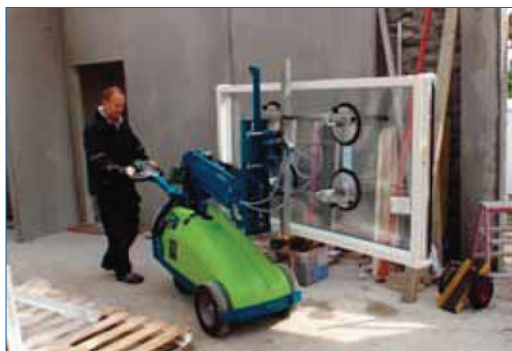
The Winlet 350 can transport heavy glass and windows, and is narrow enough to fit through a standard doorway.
