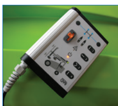
Wired remote control allows accurate placement of materials
