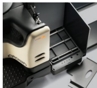
Battery Roll-out System
